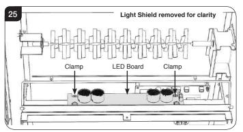
13.3 Push the rear clamp towards the rear of the firebox to release the board, see Diagram 26.
