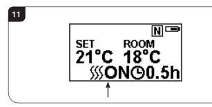
Note: It is normal for the fan heater to stop running for periods of time. This happens if the room temperature is higher than the temperature set on the control.
