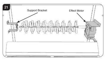
12.3 The Effect Spindle is attached to the Effect Motor by a rubber sleeve.
