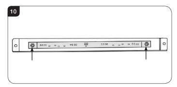
5.5 Disconnect the wire from the LED board.
