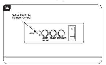
Resetting of the remote control is necessary if the appliance operates incorrectly due to external interference signal and the remote control is not in use.
