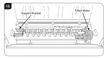
9.3 The Effect Spindle is attached to the Effect Motor by a rubber sleeve.
