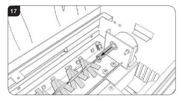
9.4 Withdraw the spindle from the left hand bracket, see Diagram 18.
