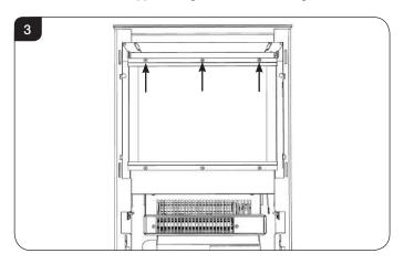
3.5 Carefully tip the glass forward and lift out of the bottom bracket to remove. Place carefully to one side.
