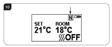
2b.25 Press the '+' or '-' button to adjust the setting temperature from 17 °C to 25°C.
