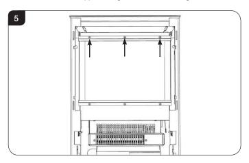
4.4 Carefully tip the glass forward and lift out of the bottom bracket to remove. Place carefully to one side.
