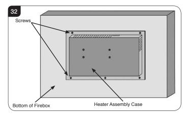
16.3 Remove the 4 screws from the front of the heater casing, see Diagram 33 to free the heater assembly.
