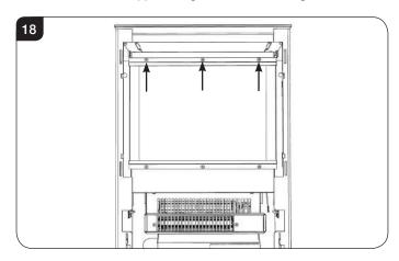
3.9 Carefully tip the glass forward and lift out of the bottom bracket to remove. Place carefully to one side.
