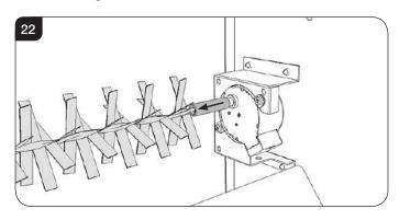
12.4 Withdraw the spindle from the left hand bracket, see Diagram 23.
