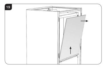
Note: When refitting the glass ensure that the top and bottom glass seals are in position on the glass. The bottom seal may remain in the bottom bracket, if this occurs it will be necessary to carefully extract the seal and centrally reposition on the bottom of the glass before reinstalling.
