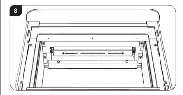
5.3 Carefully lower the LED Light Bar and disconnect the cable from the right hand side, see Diagram 9.
